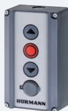
Push button DTH RM For separate control of both operational directions, with separate stop button. With miniature lock: Operator is deactivated. It is not possible to move the operator (2 keys included in the scope of delivery). Protection category: IP 65 Dimensions: 90 × 160 × 55 mm (W × H × D)
